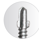
Wings to cut clearance hole means no sheet ride
